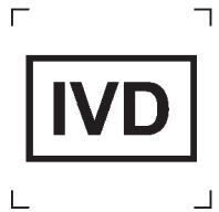
Figure 5. Symbol of in vitro diagnostic (IVD) medical devices, see SFS EN ISO 15223-1.
